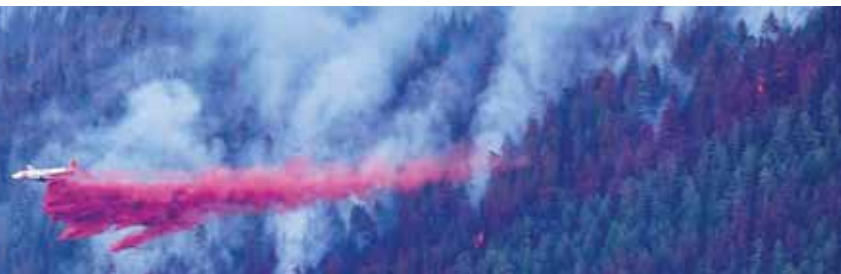
A DC-7 dumps 3,000 gallons of retardant on an area already painted red with the stuff to try to keep the fire on the left from moving to the right (south) overnight.
