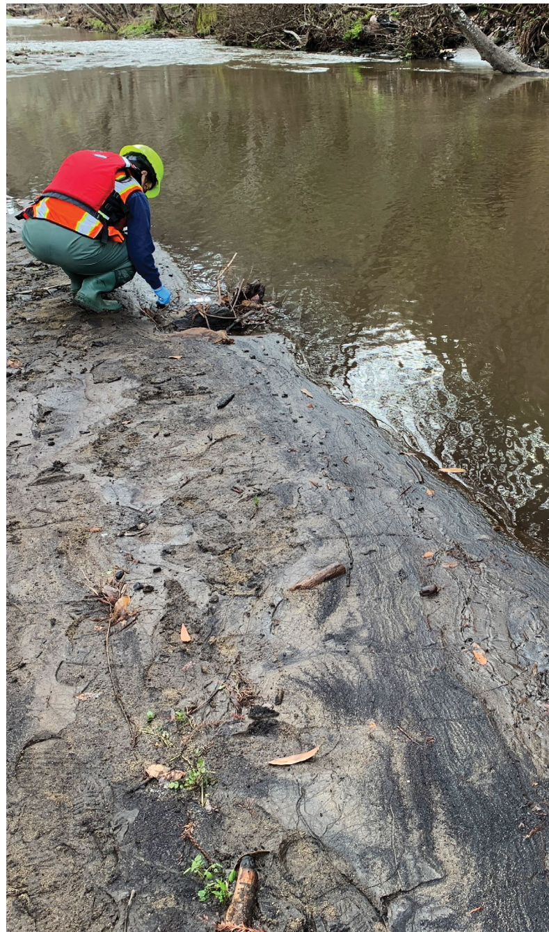
Downstream from California’s massive CZU Complex Fire, Research Geologist Renee Takesue samples stream sediment in the lower parts of burned watersheds to measure contaminant concentrations following major storm runoff. (U.S. Geological Survey photo by Amy East).
