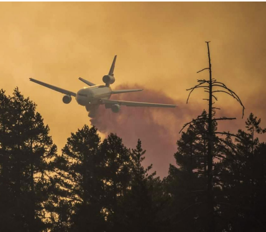
Flying out of Medford Air Tanker Base, a DC-10 very large air tanker drops fire retardant (Forest Service photo).
