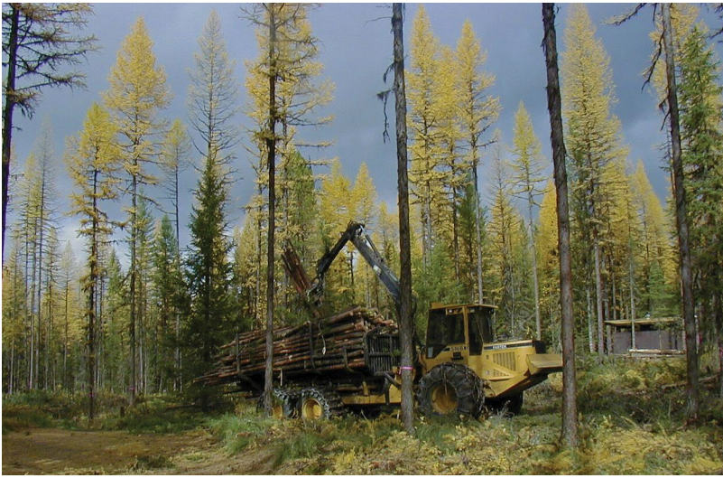
A forwarder stacks logs on the Flathead National Forest in 2019 as part of a thinning project encouraged by Trump administration policy. This type of heavy equipment in forests has been shown to damage sensitive soils and spread invasive weeds that exacerbate wildfire risk and damage forest health (Forest Service photo).
